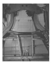
**Seat Belt Mounts:** MGA 1600MK II frames have seat belt mounts welded to them. We can weld these mounts to any frame if desired.
